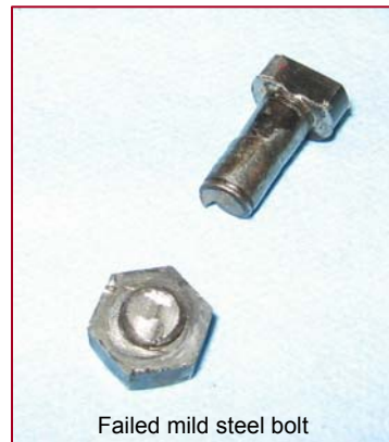
Second bolt with damaged head
